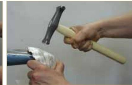
Do not clench the handle in a white-knuckle grip like this. Also, it is usually better to hold the handle closer to the end rather than choking up like this.
