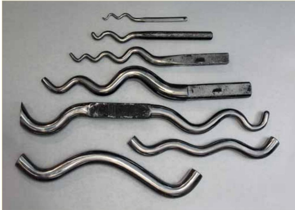
A full collection of steel sinusoidal stakes. This is more than a beginner would need, but having this wide range of sizes allows forms in almost any scale.
