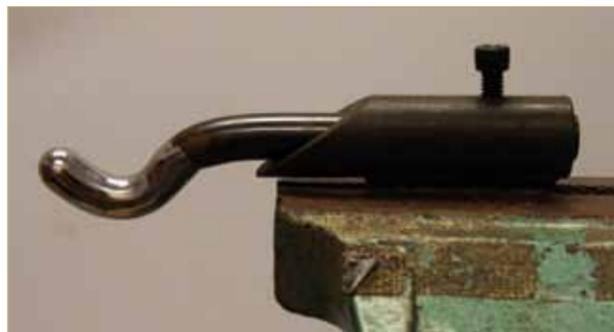
An end-hook stake in a holder designed and made by Michael Good, clamped into a vise.
