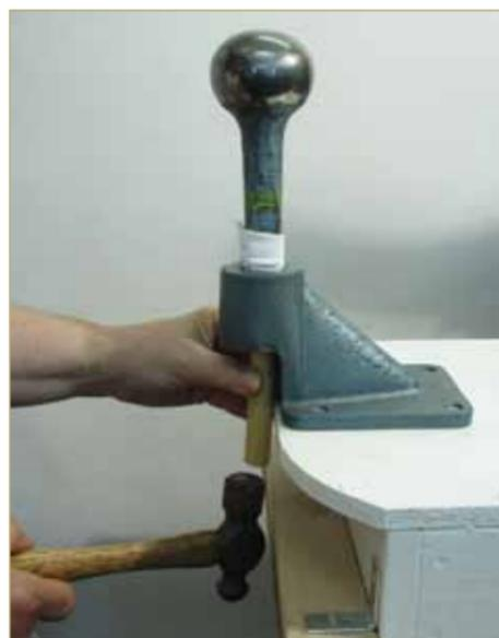
Use a piece of straight steel or dowel rod to hit the shank of the stake upward from the bottom. This reaches into the holder and doesn't damage the hammer.
