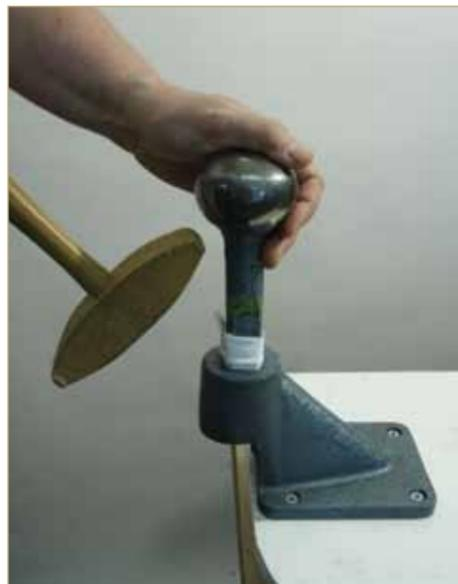
When a stake is difficult to remove from a stake holder, loosen it by tapping with a mallet at a diagonally upward angle.
