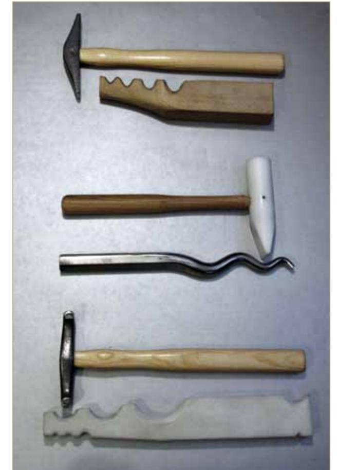
Typically, a steel tool is matched with a plastic one—use a steel hammer on a plastic stake or a plastic mallet on a steel stake. Metal on metal allows for faster forming but risks thinning and denting the form.
