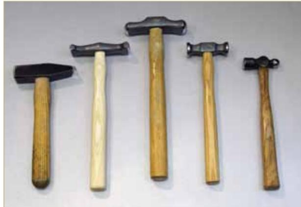
Basic shapes of steel hammers. From left to right: Forging, raising, forming, planishing and ball peen.
