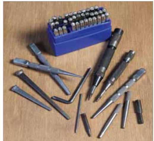
Familiar tools like these can be used as texturing stamps, often without any modification.
