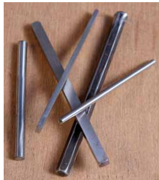
Tool blanks come in many sizes and shapes.
