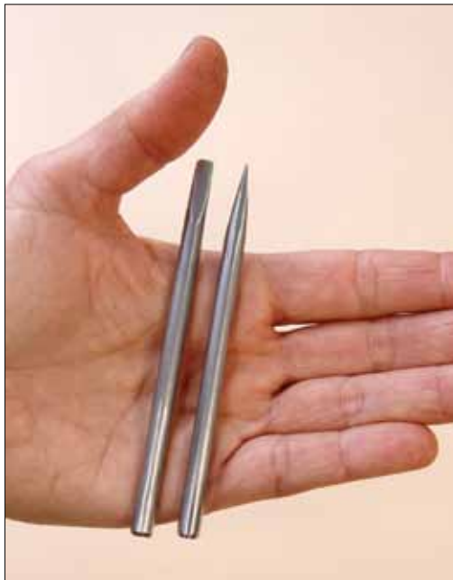
Liners are perhaps the most frequently used of all chasing tools. They are equivalent to pencils on paper for making lines, patterns, and textures.
