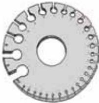
To use a gauge plate, find the slot that makes a snug fit, but don't distort the metal by jamming it in. Be careful not to measure where the edge has been thinned by planishing, or thickened by shears.
