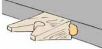
Avoid drilling holes in the bench pin because they trap metal and eventually make the surface irregular. Keep a block of wood handy for drilling. An exception to this is a few well-placed holes that make it possible to work on objects with pinbacks and similar projections.
