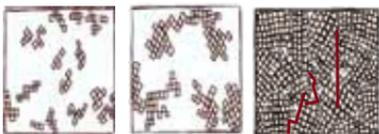
As crystals form, they bump into one another, forming irregular grains. The red line traces grain boundaries.
