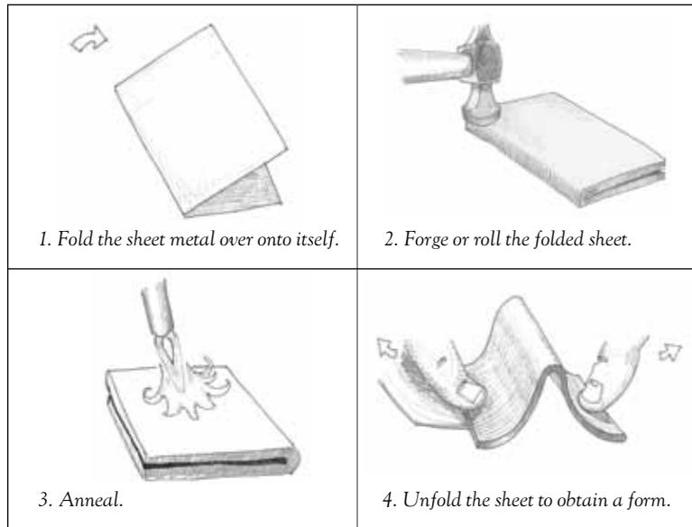
Principal variations include the style of the fold, the number of folds, and the ways a series of folds react to each other. Some types of foldforming (scoring and bending, for instance), involve setting up a weaker place in sheet metal so that the metal will bend or fold on a specific line. Other avenues of related folds include interwoven and tube folds.
