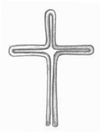
*Cross-folds are made by creating a structure with the cross section of a cross, or plus sign: +. In this example, two folds have been made, the second running at a right angle to the first.*
