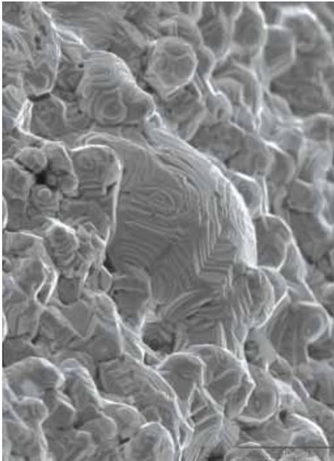
*At even higher magnification, each silver particle shows the crystals of which it is made.*
