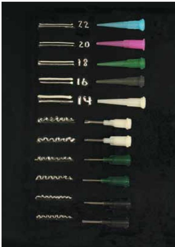
The upper line in each example is the unfired extruded line, which is roughly the size of the B&S gauge number shown beside it (made with the syringe, of course). The lower line has been fired and is a bit smaller as a result.
