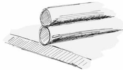
To build a bezel, lay down a single syringe line, allow it to dry, then lay another on top of the first.
