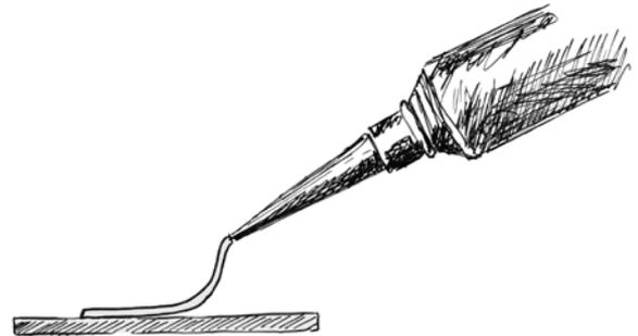
The syringe should hover about a quarter of an inch above the work, allowing the thread to drop down into position. Touch the tip to the work to start and to terminate a line.
