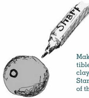
Make a core from a combustible material such as paper clay, cork clay, or Styrofoam. Start by marking the location of the holes with a marker.
