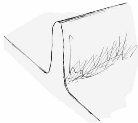
When the bezel wall has dried, lay thick slip along the wall to create an even surface. Smooth with a damp brush as needed, dry, then sand.
