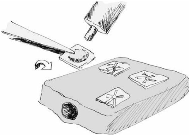
To apply ornamental elements, pre-fire them, then place a dab of syringe on the back of each piece and press it onto the glass. Fire at 1200° F (650° C).
