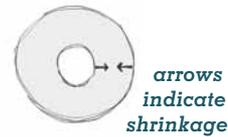
This drawing shows how shrinkage will affect a PMC ring. The silver parts will shrink, but the center hole will not—it is made of air, which doesn’t shrink. The ring will be smaller after firing than it was before, but the hole will be about the same.
