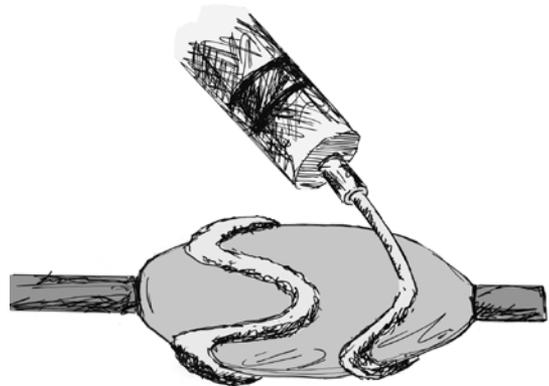
Syringe PMC can be applied to glass, for instance a bead like this. If you don't know the melting point of the glass, you should experiment to be sure it is compatible with PMC. If possible, use wavy threads, which will allow for shrinkage.
