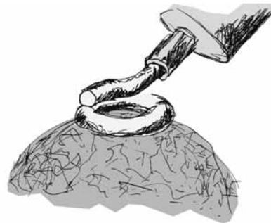
Extrude a ring of PMC around the mark. Allow it to dry, then flow another ring on top of the first. Depending on the design, these rings can be refined or not.
