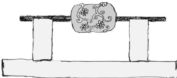
Fire glass or ceramic beads on a rack or stilt of some kind. These are commercially available, or you can use a piece of nichrome wire suspended between a couple pieces of soldering board or posts.
