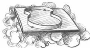
7 Set small pieces of solder against the bezel so they are in contact with both the wall and the base. If you plan to cut away the metal around the bezel, put the solder on the outside of the loop. If not, put the pieces on the inside.
