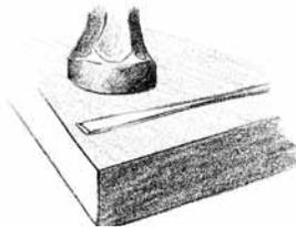
3 Bend the loop to fit the object, either by eye or by bending it around the piece itself. The wire will always spring back, so go past the joint to allow for this. Check against the object periodically as you work to make a perfect fit. Fussiness at this point will make a better looking bezel and an easier setting job later.
