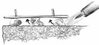
9 When the solder flows, immediately pull the flame away. Allow the piece to cool for a few seconds, then quench it in water. Examine the joint, and if it is complete, put the piece in pickle to remove flux residue and oxides.
