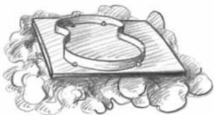
6 Clean a piece of metal that will be the base, and apply a layer of flux. Lay this on a bed of pumice pebbles rather than setting it flat onto a soldering block. This will allow heat to surround the sheet and let it heat up faster. Set the bezel into position and slide it back and forth to transfer a film of flux onto the walls of the bezel.
