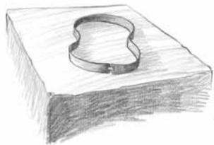
5 Check the fit by pressing the bezel onto the object. In the process, be careful that you don't distort the wall. It must remain vertical. Rub the bezel on sandpaper so the bottom edge is flat.
