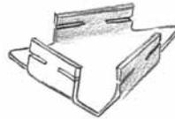
4 Set the object in place and bend the tabs sideways to lock the piece in position.
