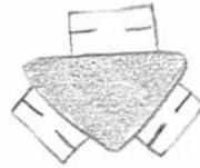
3 Cut the metal to the proper shape, solder on additional parts (if necessary), and finish with patina, polish, etc. Bend the tabs upward, here to a 90° angle.
