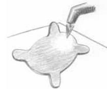
5 File and sand the edges, solder parts such as bails or accents if they are needed, and create the intended finish
