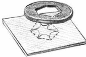
3 Transfer the pattern to metal. Drill access holes to allow for inserting a sawblade, and cut out the tabs.
