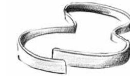
4 When the fit is assured, snip the end and solder the loop closed. Use only a tiny piece of solder—first, because we don't want a silver blob on the copper bezel, and second, because solder is stiffer than copper and a bulge of solder will be difficult to press down during setting.
