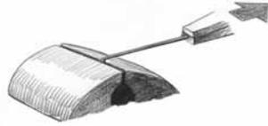
2 Planish the wire with a polished hammer. If the wire curves, it is because the hammer blows are not landing squarely. Adjust as needed. Snip and file one end of the wire to make a square end.
