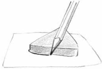
2 Figure out where the tabs will be. In many cases, as in this example, the tab will first bend up vertically to make a wall that will hold the piece from sliding side to side. Layout the lateral tabs, typically by making a single saw cut (A). It is a good idea to test the idea on stiff paper.
