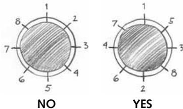
At this point the object should be gripped in place, though the bezel looks rather unattractive. Continue the process, starting midway between two cinches, and again jumping across the form for the next push. As the process continues, the waves of the bezel get progressively smaller until they are completely smoothed away.
