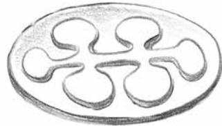
2 If there is work to be done on the base piece (there usually is), do this first. This would include things like soldering on pin findings, bails, or other attachments. The idea is to get these parts properly located first. Drill holes in the base piece where they will not be in the way of other parts of the piece, such as the pin finding.
