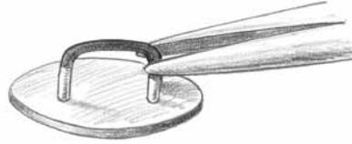
5 Check the soldered joint to be sure it is solid. If there is a fillet at the base of the pin, file it away so the staple will rest securely against the base.
