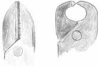
The shape at the left is called a wire cutter, side cutter, or snip. They are sold in many sizes, and should match the scale of work you do. The tool on the right is called an end cutter.
