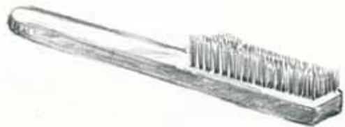
*Whether steel or brass, lubricate the burnishing action with soap and water.*
