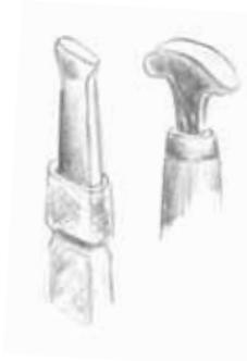
*A toothbrush handle and a traditional steel bezel roller are other tools used to press a bezel over a stone.*
