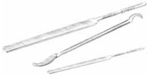
Needle files, rifflers, and escapement files are useful for delicate shapes and surface adjustments.
