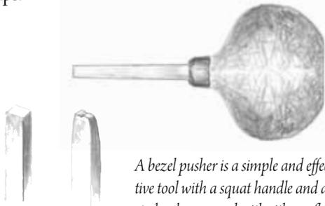
*A bezel pusher is a simple and effective tool with a squat handle and a steel or bronze rod with either a flat or notched face.*
