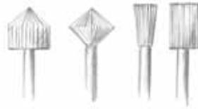
*These are the most common burs used in stonesetting. From left to right: setting, Hart, inverted cone, and cylinder.*
