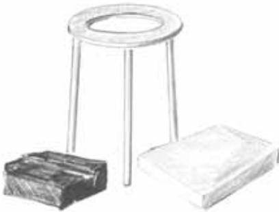
*Three time-tested soldering surfaces are a charcoal block, a soft firebrick, and a steel tripod, usually used with a screen on top.*
