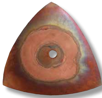
Mustard on copper, sealed under a container to fume for 24 hours, removed with hot water.
