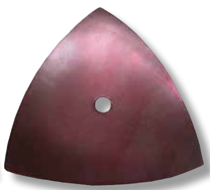
Copper in the oven; 350° F for 20 minutes.
