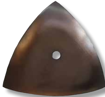
Liver of sulfur on copper.
