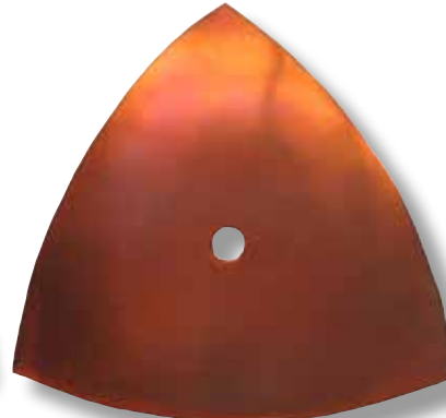
Copper in the oven; 300° F for 30 minutes.
