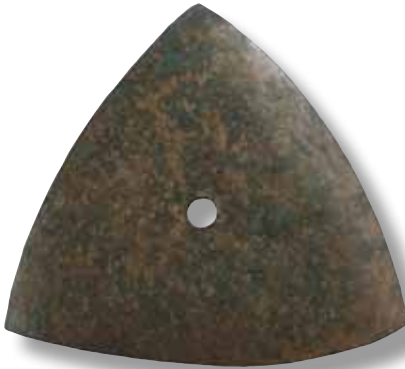
Ammonia / vinegar in pine sawdust on copper.
