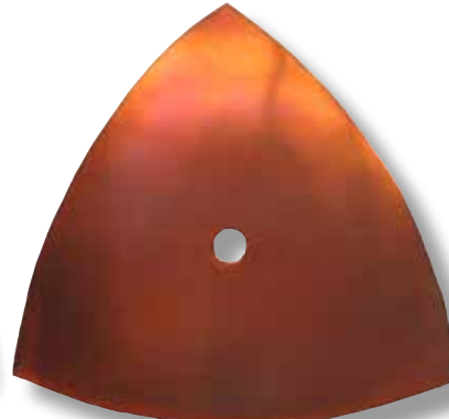
Copper in the oven; 300° F for 30 minutes.
