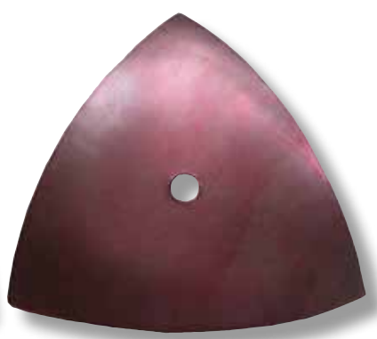
Copper in the oven; 350° F for 20 minutes.
